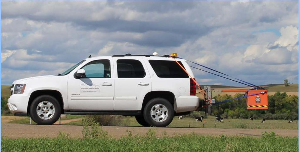
GSSI 1-GHz Horn Antenna
